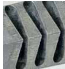
Microprocessing of cobalt-based carbide 200 \mu\text{m}
