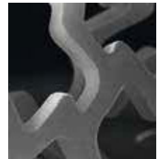
Cutting of coronary stents 100 \mu\text{m}
